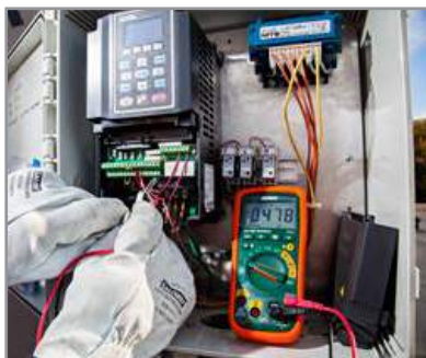
Low Pass Filter (LPF) ensures accurate AC Voltage measurements on a variable frequency drive.
