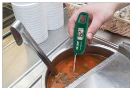
2.4" (61 mm) folding stainless steel probe (NSF certified) for measuring in liquids, pastes, and semi-solid food. Ideal for use in food industry, agriculture, and laboratories.
