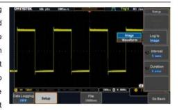
data in CSV file. Data can be saved to USB, GDS-1000B or remote computer via LAN. It is very user-friendly and also an advanced measurement management tool.
