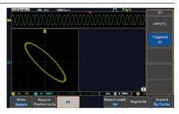
For engineers working for the industries, the X-Y mode display can be used to conduct yield rate tests for basic components' electric conduction and non-conduction. Therefore, the X-Y mode display plays an important role in basic oscilloscopes.
